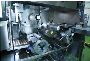
blisters per minute thus making production much faster. However, the OEM had challenges with controlling the temperature which is a critical aspect of this machine because sealing is dependent on effective temperature control. If the temperature is not controlled properly then the quality of final blister would be bad & it won't be sellable in the marketplace.
